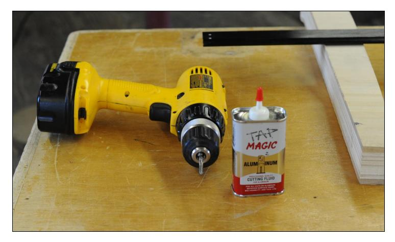
The easiest way to cut threads is with a tap in a battery powered drill. The tap size is  $4.0\ x$  .7mm.
