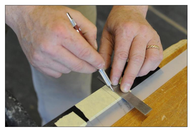
The treble end of the rail is  $10\,\mathrm{mm}$  or about 3/8'' from the tray flange line. Mark the tape with this measurement.
