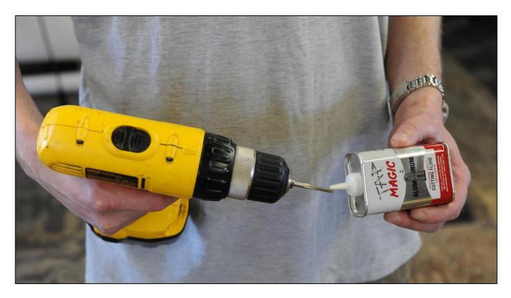
Cutting threads in aluminum is easy however, you will need to apply cutting fluid to the tap. The cutting fluid keeps the aluminum from balling up in the threads causing a stripped hole.
