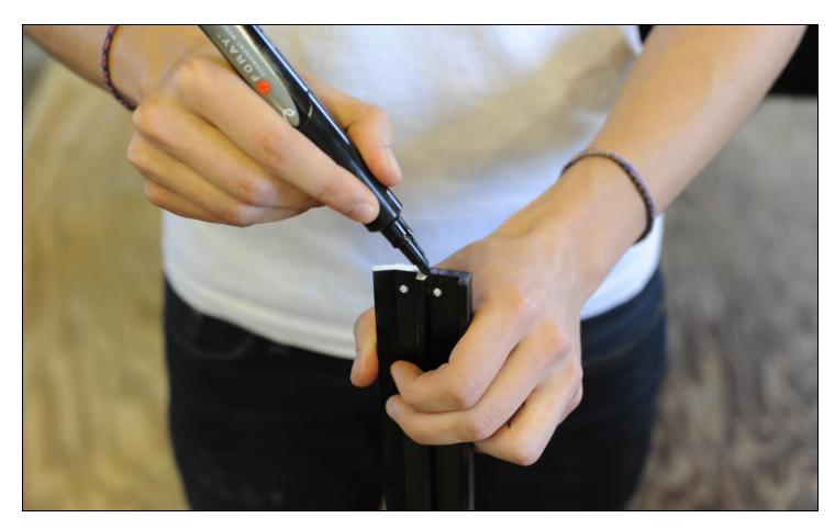
You can use any kind of felt tip to black in the end of the rail. A paint felt tip works the best. Obviously the color choice should be black.
