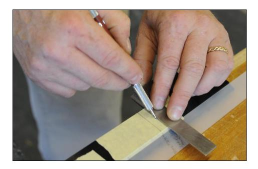
This line should be on your damper action scale stick. The end of the rail will be  $10\,\mathrm{mm}$  or about 3/8'' from the treble Tray Flange.
