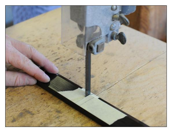
Use a bandsaw to cut the flange rail to length. Cut to the outside of the line you marked on the tape. You can also use a hack saw if you wish.
