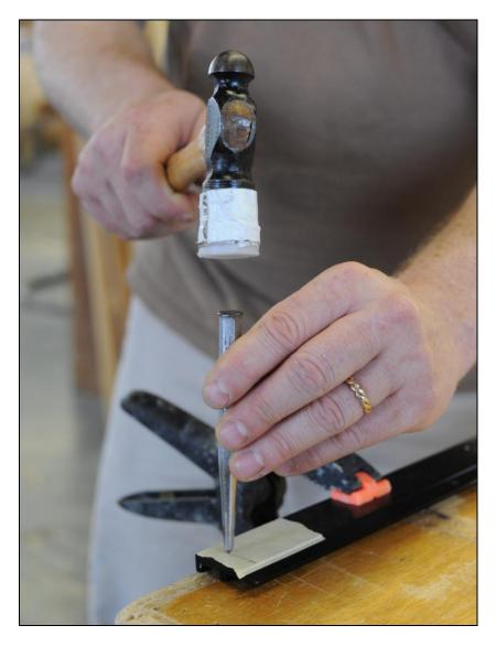
Place the tip onto the intersection of the lines on the tape and strike the punch with a non metallic hammer. This operation is necessary for the punch mark to reliably hold the drill bit when drilling.
