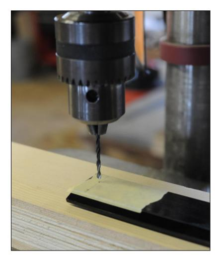
Put a 3.3mm drill bit in the drill press. Note that this is the same drill bit used for the flange screws.
